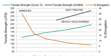
Amount of Tubing Reduction (i.e. increasing cold work)
