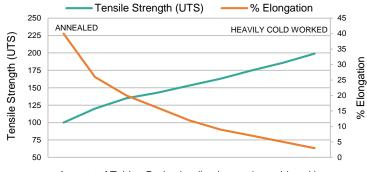
Amount of Tubing Reduction (i.e. increasing cold work)
