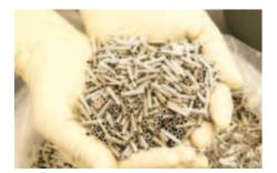
Cleanliness of stainless steel parts is becoming increasingly important to medical device and other manufacturers. Problems caused by inadequate or improper cleaning can result in increased process costs for fabricators of metal tubing.
